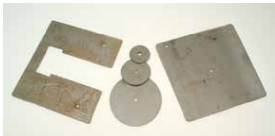
Photo #1.15 (Weight materials must be painted and the weight of each piece clearly marked)
