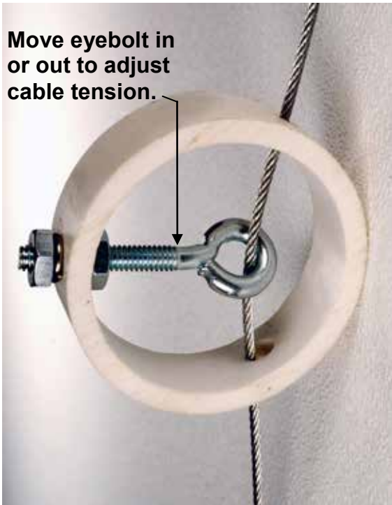
Photo #11.9(a) (Cable Adjuster Assembly)
