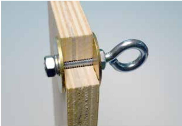
Photo # 8.12 (Eyebolt will face rear of car)
